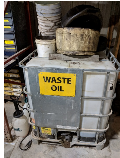
12) Mislabeled used oil storage container
